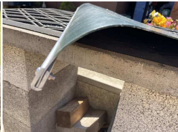
Strengthening aluminium moulding on the side of the bonnet.
