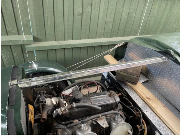
Mock up of hinge assembly. Details of aluminium angle hinge strengtheners (before final fettling).
