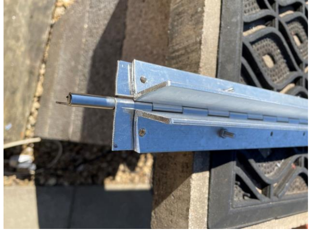
Mock up of hinge assembly. Details of aluminium angle hinge strengtheners (before final fettling).
