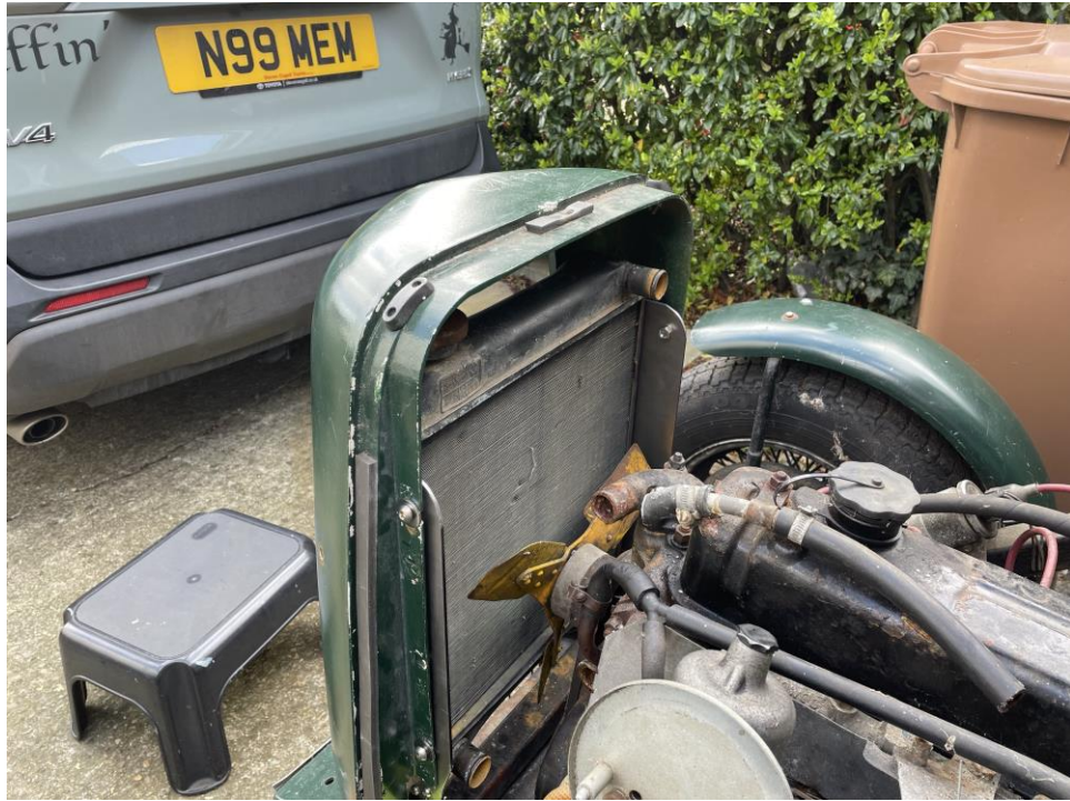
Trial fit with the Land-Crab radiator and new brackets.
