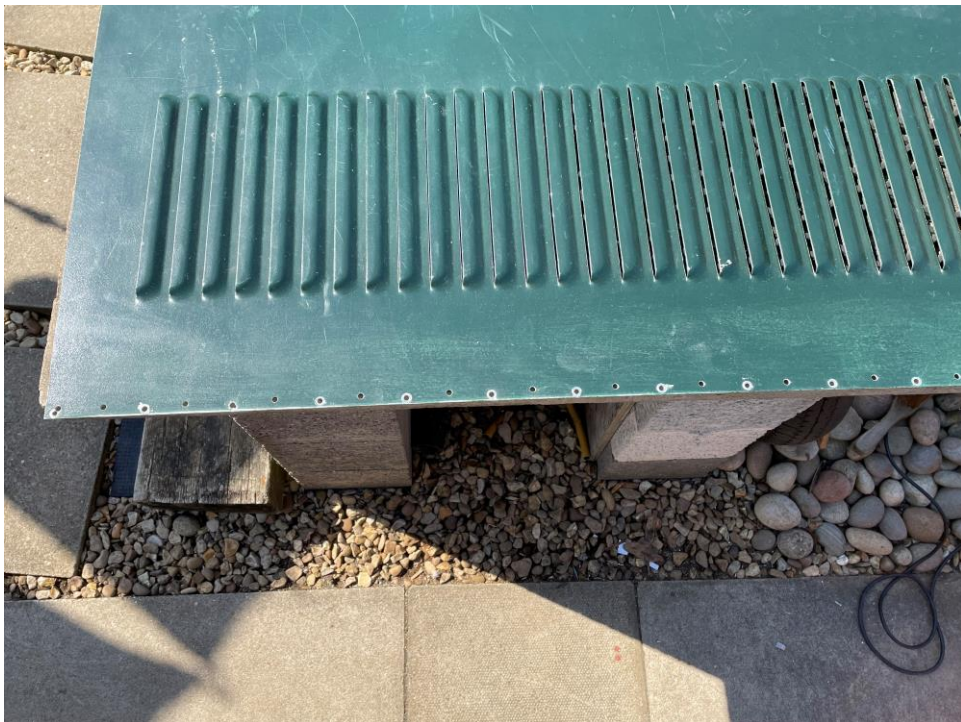
Old and new holes in the side panel.
